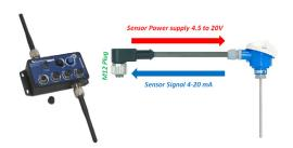
The sensor is directly powered by a high accuracy and adjustable DC/DC converter integrated inside the device. The excitation voltage is remotely configurable through the BeanScape® (4.5 to 20V).
